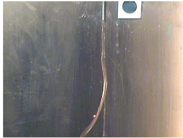
Fig. 3. The unstable and asymmetrical rivulet flow on the copper plate with M = 0.003825 , i.e., the third plotted point in Fig. 12. The picture shows the laser beam star and the black circle as the benchmark of a linear dimension.
