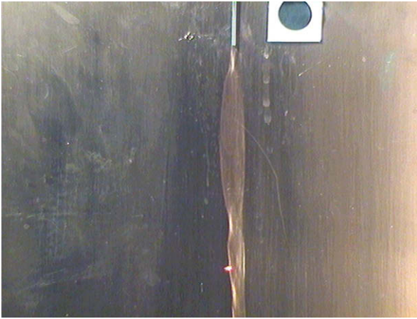
Fig. 4. The asymmetrical rivulet flow on the copper plate with M = 0.008197 , i.e., the last plotted point in Fig. 12.
